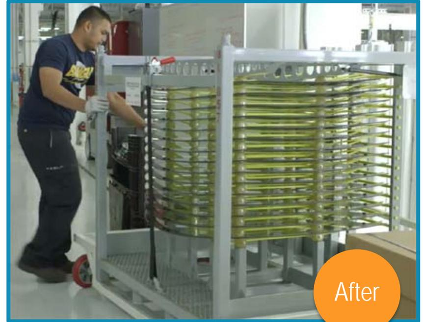
**After:** Switched to custom-made, reusable racks for shipping windshields, with help from a \$30,000 StopWaste grant. The returnable racks are walked straight to the production line.
