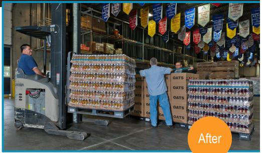
**After:** Switched to plastic pallets, replaced shrink wrap with thick rubber bands long enough to fit around a pallet and secure products.
