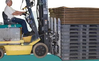
Gatorade chose pallets with an interlocking pattern that increases stacking stability and makes it easier and safer to store and transport empties.
