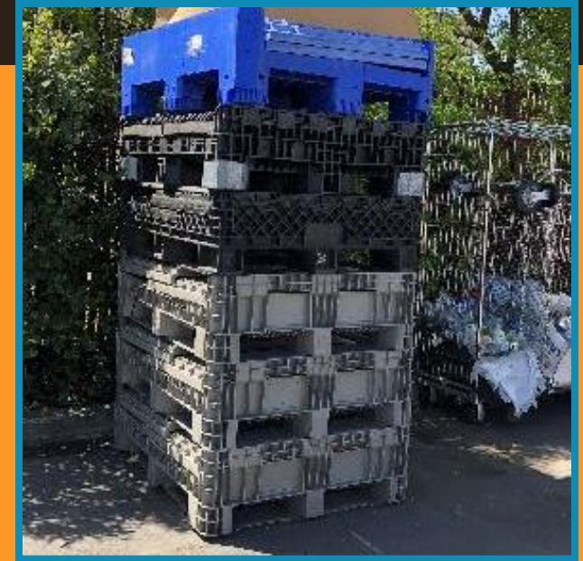
Surplus Service's new plastic bulk containers are reusable and collapse for space-efficient storage. Pictured above: 6 collapsed and stacked bins.
