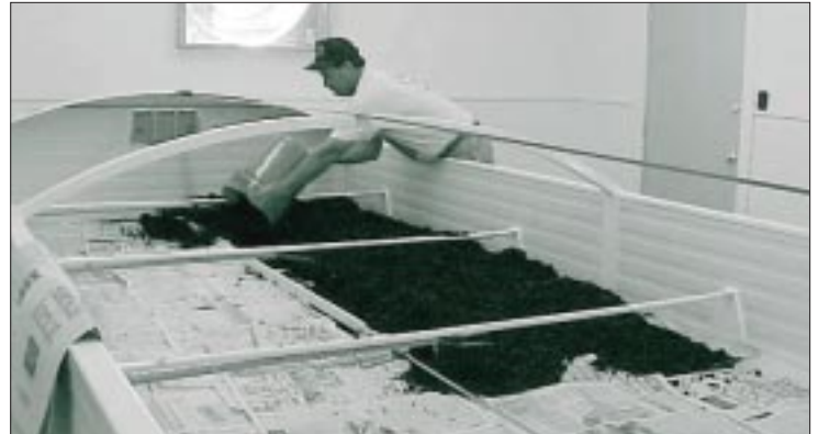
Thousands of worms live in the Vermitech Systems composting digester at MUSC, turning food waste into a valuable soil amendment.
